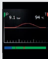
Once the desired temperature profile has been set for a dose, it is possible to check during a coffee dispensing, that the extraction temperature follows the chosen profile and that the quantity of the dose dispensed is the correct one, all without waiting for the end of the brewing but in real time. Coffee brewing becomes a real-time dialogue between barista and machine, with the aim of increasing human-machine interaction to achieve the best product in the cup.
